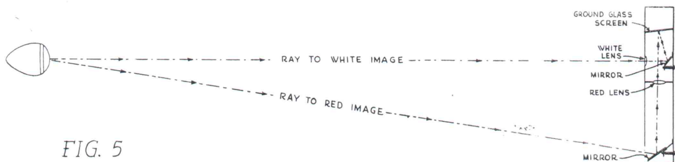
Diagrammatic cross section showing how the Optoscope works
